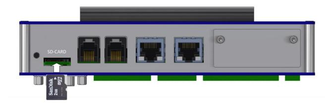
The SD card interface operates in accordance with the Push-Push principle, i.e. the card is inserted into the slot and latched into place with a light push. Another push on the card unlatches it and allows it to be withdrawn again.
